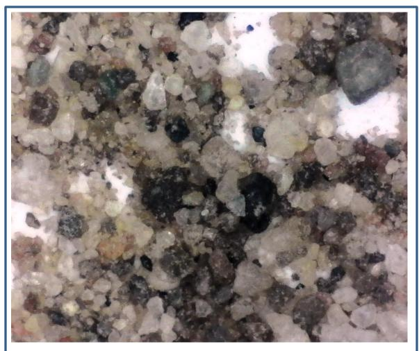
Poorly sorted, mixed beach sand. There is quartz, but also carbonate rock fragments and even some silt/clay. FOV ~ 5 mm.
